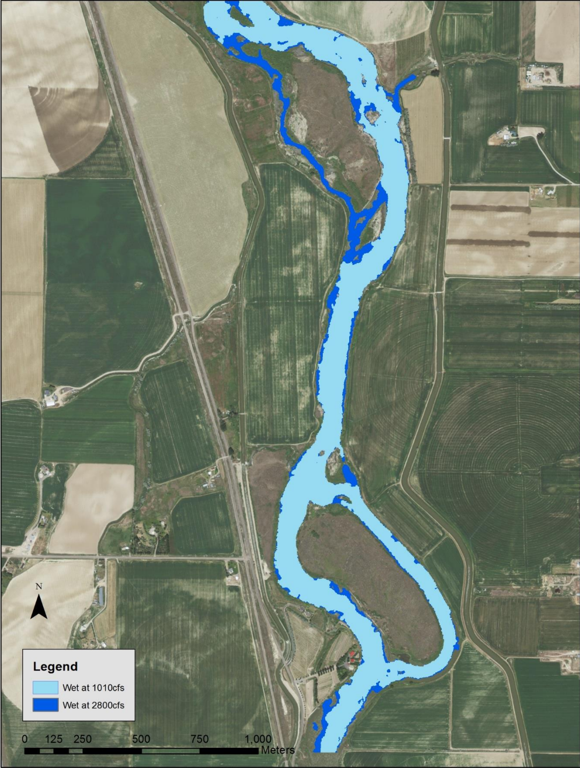
Figure 1b. Osgood Reach of the Snake River, south half, showing comparison between wetted perimeter at 1,010 and 2,800 cfs.
